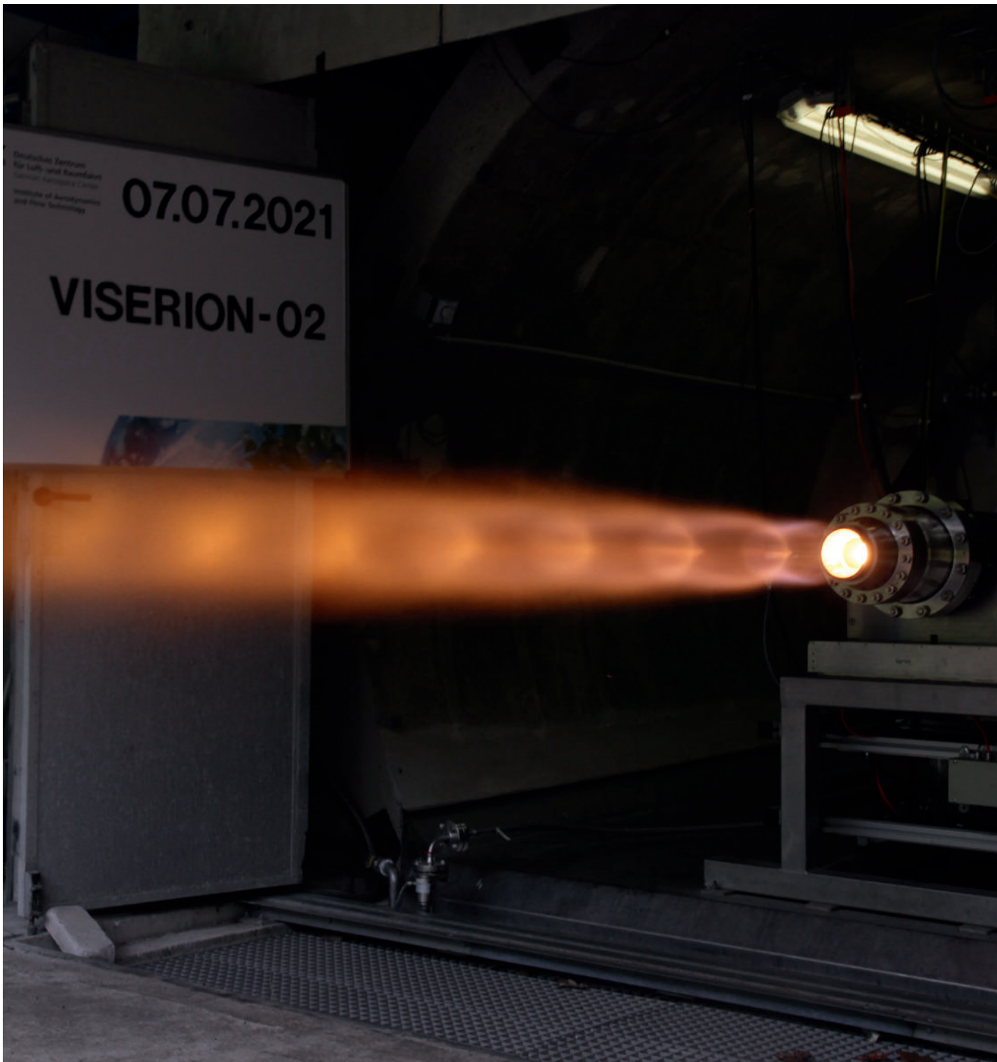
The German Aerospace Center (Deutsches Zentrum für Luft- und Raumfahrt, DLR) successfully tests the VISERION hybrid rocket engine using Evonik's highly concentrated hydrogen peroxide, PROPULSE®.
