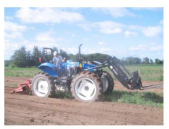
Figure 4: Incorporation of DARAMEND into soil using specialized tillers.
