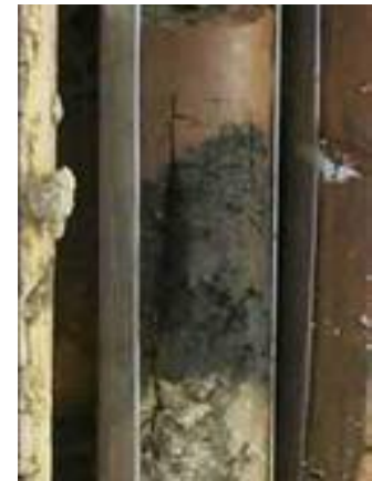
Figure 2 - EHC layer injected between clay and weathered limestone
