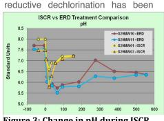
Figure 3: Change in pH during ISCR and ERD pilot tests
