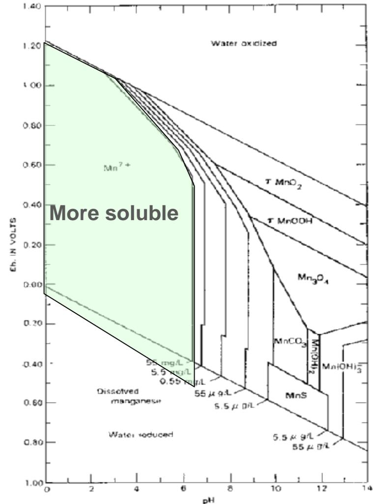
**Figure 16.** Fields of stability of manganese solids and equilibrium dissolved manganese activity as a function of Eh and pH at 25°C and 1 atmosphere pressure. Activity of sulfur species 96 mg/L as SO<sub>4</sub><sup>2-</sup>, and carbon dioxide species 61 mg/L as HCO<sub>3</sub><sup>-</sup>.
