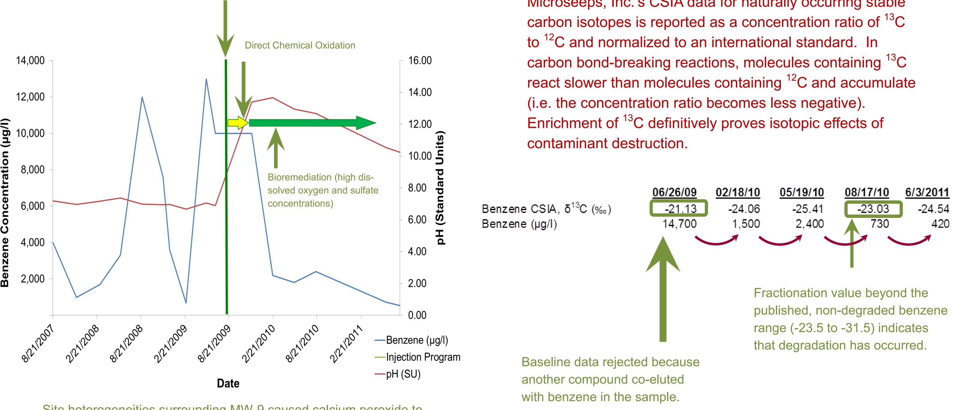
Site heterogeneities surrounding MW-9 caused calcium peroxide to accumulate and locally increase pH. pH in the MW-9 area became more neutral as calcium peroxide elutes oxygen and is depleted. However in the winter of 2011 the well was replaced by MW-9R located directly adjacent to MW-9. pH in MW-9R was neutral.
