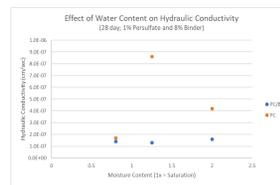
Water content should be included as a design parameter for ISCO-ISS projects "from bench to field" to maintain predictable UCS results.
