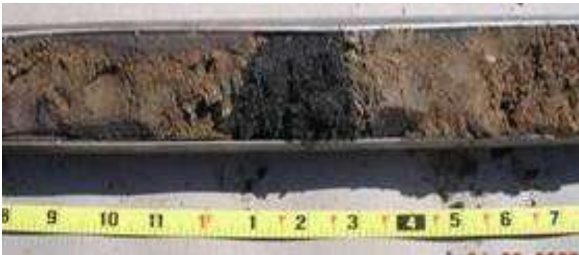
Horizontal EHC fracture.
