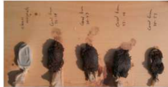
Figure 3. Iron collected during coring of 33'-38', 38'-43', 43'-48' and 48'-53'. A clean magnet is shown for comparison.
