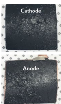
Photographs of the opened cell after formation: Composite gel polymer electrolyte is clearly visible
