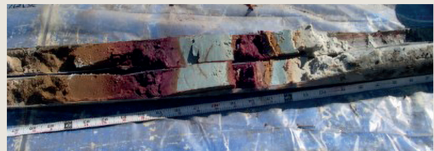
Soil core from a site in Gainesville, Florida treated with ISGS® TECHNOLOGY.
