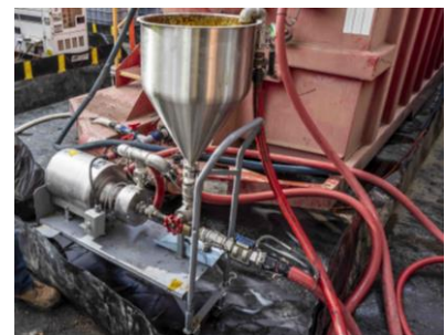
Figure 2 | In-line emulsifier pump with Venturi induction system
