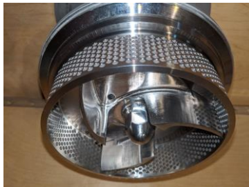
Figure 5 | Shear head designed for efficiently creating an emulsion from ELS Concentrate.
