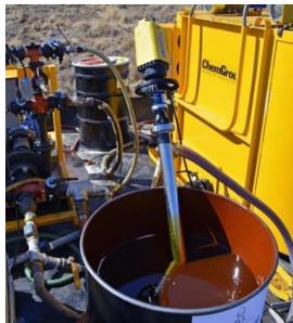
Figure 4 | ELS® Liquid Concentrate drum and transfer pump
