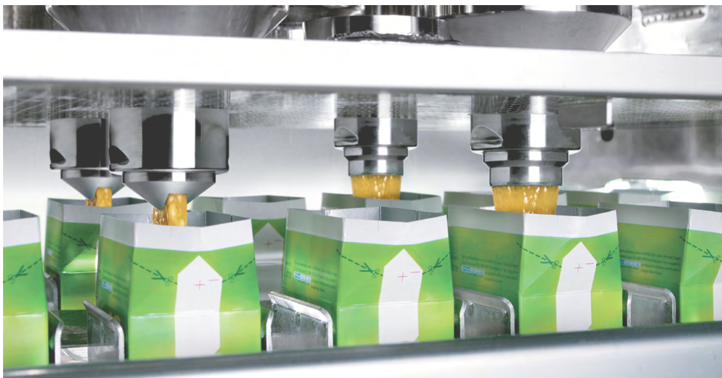
Aseptic food packaging machines sterilize, form, fill, and seal the package under aseptic conditions.
