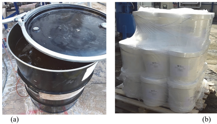
Fig. 4. ELS ® Microemulsion barrel (a) and pails with the EHC ® Liquid Mix compound (b)
