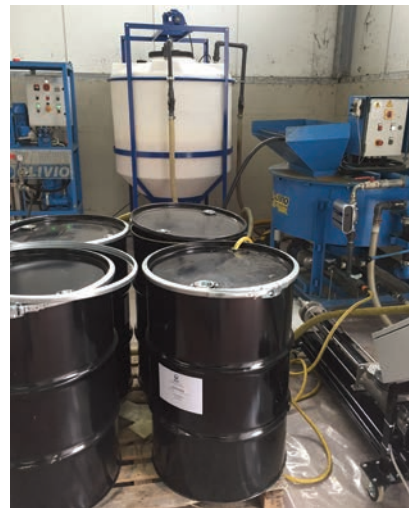
Fig. 7 - Pre-mixing tank (on the right) and final mixing tank with in-line recycling system (in the middle).
