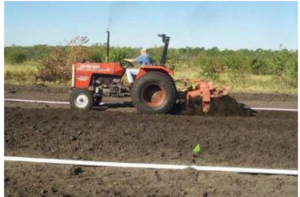
Figure 1: In-place application of Daramend Reagent
