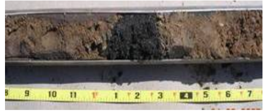
Horizontal EHC fracture
