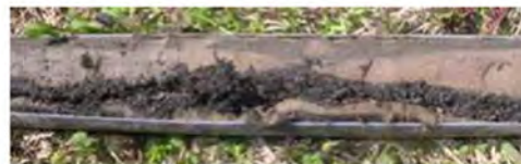
EXHIBIT 5 Injection set-up and soil verification borings showing EHC material emplaced in discrete bands (darker material)
