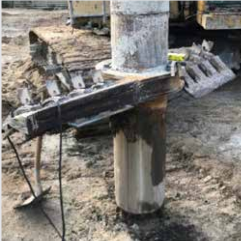
Figure 2. Mixing head with one level of flights designed to mix the soil in situ
