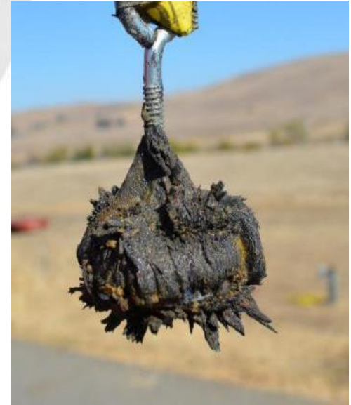
Microscale ZVI on magnet collected from inside monitor well after injection
