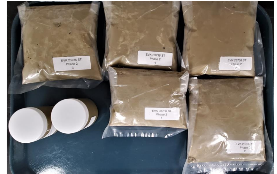
Tedlar bags set up for shipment to accredited lab for soil analysis and cylinders for leach testing and UCS analysis
