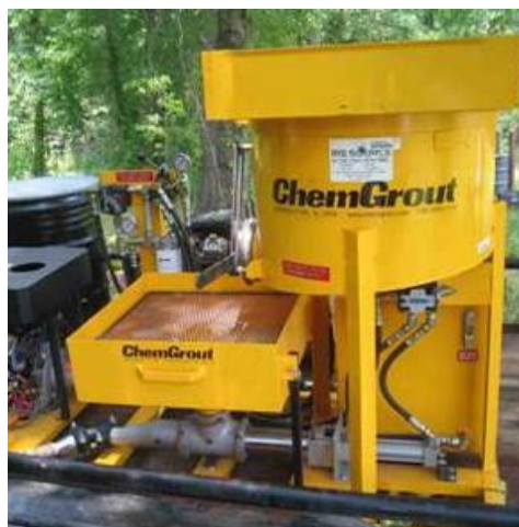
Figure 7. Grout / paddle mixing unit with feed-tank and injection pump.
