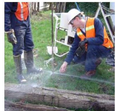
Figure 2. Low pressure water test of pressure activated tip with 4 horizontal openings
