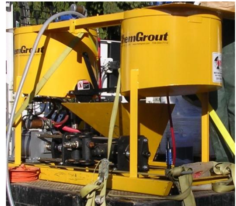
Figure 1. ChemGrout's CG-500 mixing unit with high pressure piston pump
