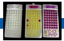
Disinfected samples are tested against controls. Both negative controls and untreated samples are shown for E. coli, measured by Colisure in a recent pilot study.
